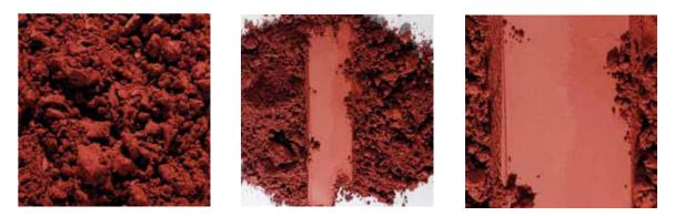
Two pigment blends, of the same shade. Right: Without titanium dioxide. Left: With titanium dioxide. The loose powder in left image shows no visual colour difference. When smoothly pressed down it shows the higher luminosity and pure color of the titanium dioxide-free formula.
